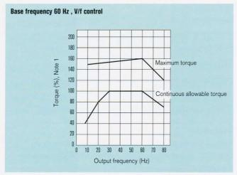
(Note 1): The 100% torque: value obtained using the synchronous rotational speed at 60 Hz as the reference. The starting torque is smaller with an inverter than with the commercial power supply Be aware of the characteristics of the load machine.
